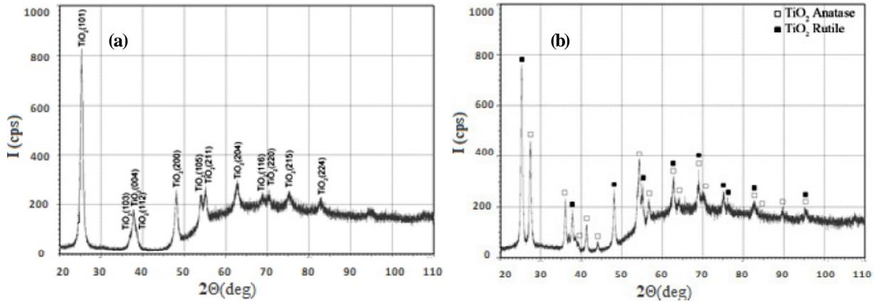
Fig. 3. X-ray diffraction data obtained for sol-gel prepared TiO<sub>2</sub> powders: sample T-1 (a) and sample T-4 (b).
