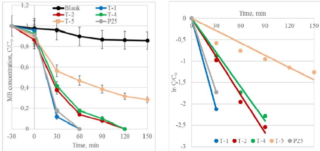
Fig. 4. Photocatalytic destruction (a) of methylene blue (initial concentration  $C_0$  of 10 mg/L) and kinetic (b) of the process.
